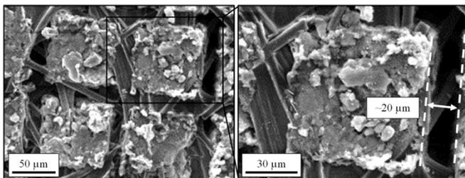
Fig. 4: Top-view SEM image of laser generated micro-grids in Cr-Ni electrode.
