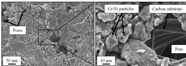
Fig. 3: Top-view SEM images of a Cr-Ni electrode surface.
