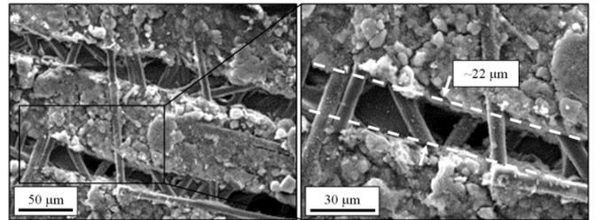
Fig. 5: Top-view SEM images of laser-generated micro-channels in Cr-Ni electrode.
