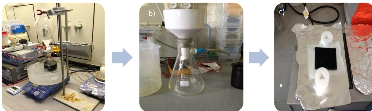
**Fig. 1:** Process flow (a) 114 ml of 5 wt%  $\text{KBH}_4$  solution was added drop-wise into the suspension at  $10^\circ\text{C}$  followed by stirring for 30 min. (b) The obtained black powder was repeatedly washed with pure water and filtered by vacuum pump until no  $\text{Cl}^-$  exists anymore. (c) This mixture was screen printed on carbon paper sample of  $5 \times 5 \text{ cm}^2$  (Quintech, TP-120-T, Toray Paper) with  $370 \mu\text{m}$  thickness.
