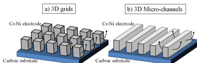
**Fig. 2:** Schematic drawing of laser-generated (a) 3D micro-grids and (b) 3D micro-channels in Cr-Ni electrodes coated onto carbon paper substrate.
