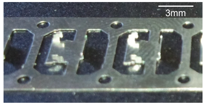
Fig. 6 Pressed products in the experiment using the small press machine.
