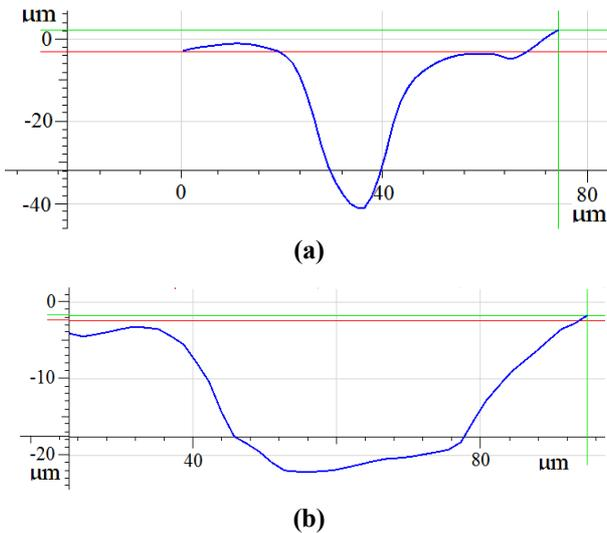
**Fig. 4: Typical cross-section profiles of best focus micro-channels machined by (a) LIPMM, and (b) Laser ablation, at a 20 kHz pulse repetition frequency and 70 mW power**
