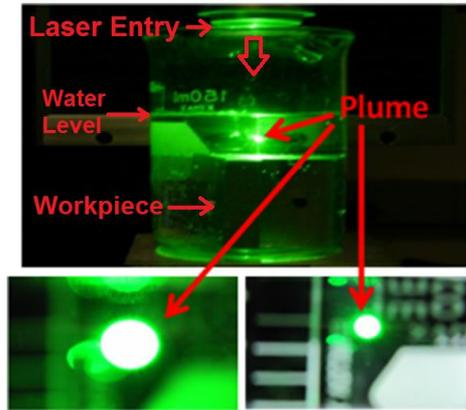
**Fig. 1: Plasma plume inside the dielectric media (beam incident from the top)**
