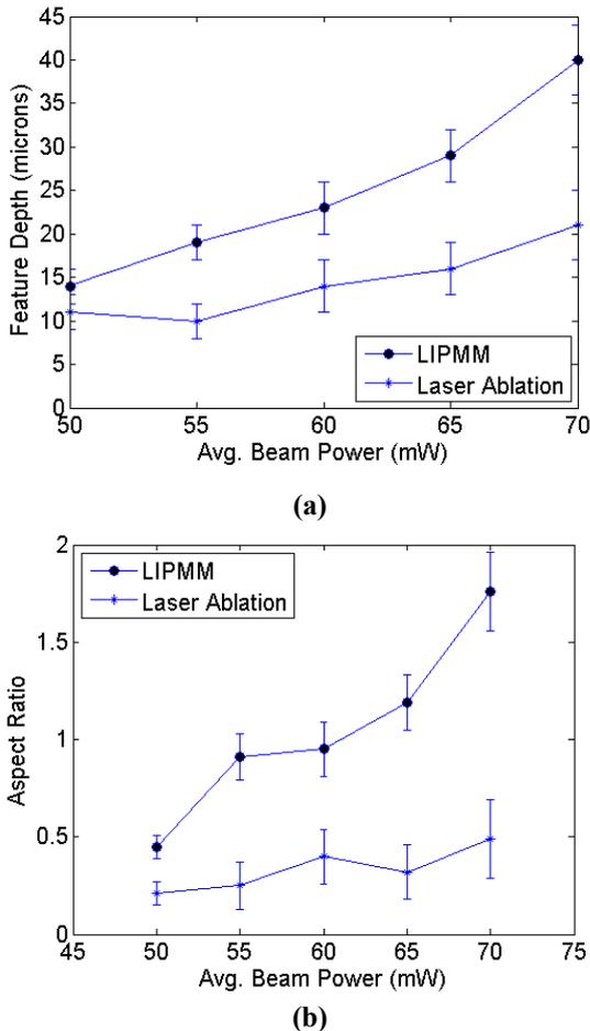
**Fig. 5: (a) Depth, and (b) Aspect ratio of best focus micro-channels vs. beam power for ABS, obtained by LIPMM and laser ablation**
