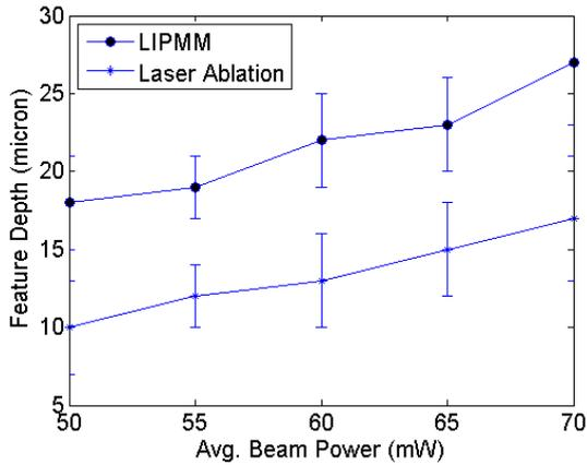
**Fig. 7: Depth of best focus micro-channels vs. beam power for LDPE machined by LIPMM and laser ablation**
