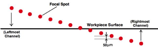
**Fig. 2: Schematic representation of micro-channel fabrication at different positions of the focal spot with respect to the workpiece surface**
