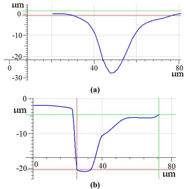
**Fig. 6: Cross-section profiles of best focus micro-channels machined by (a) LIPMM, and (b) Laser ablation, at a 20 kHz pulse repetition frequency and 70 mW power**
