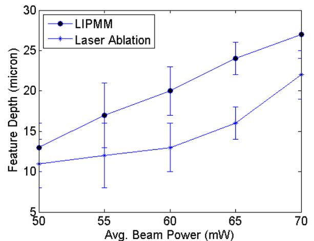
**Fig. 11: Depths of best focus micro-channels made by LIPMM and laser ablation processes at different beam powers**
