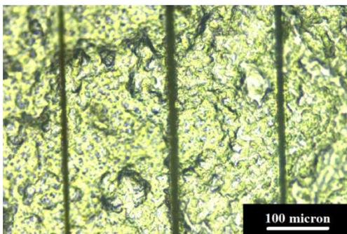
**Fig. 9: Surface image of micro-channels machined in HDPE by LIPMM process**
