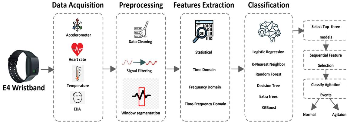
Fig. 1: E4 wristband classification system architecture.
