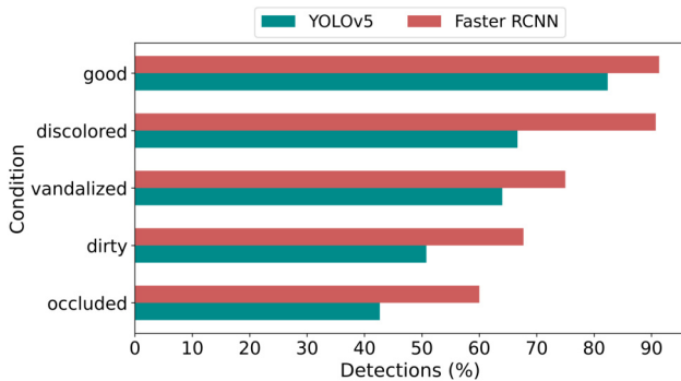
Fig. 7: Performing TSD with YOLOv5 and Faster R-CNN
