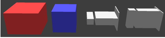
Fig. 1. The modules considered in the morphological design space. From left to right: core , brick , vertical active hinge , and horizontal active hinge .
