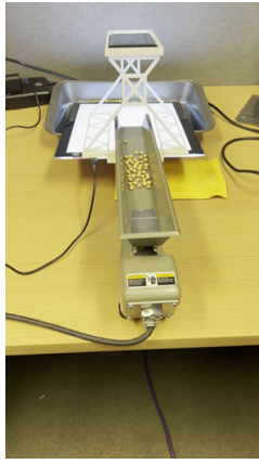
Fig. 1. Mechanical hopper delivering seed kernels
