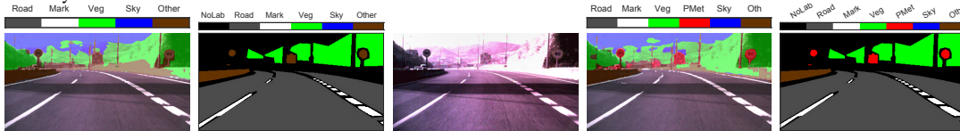
Fig. 6. Image 560 (f4, AG2, 10ms), captured during a winter, sunny morning, in road with intense contrasts: (far left) Exp2 segmentation, (left) Exp2 ground-truth, (center) false color, (right) Exp3 segmentation and (far right) Exp3 ground-truth.
