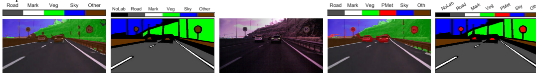
Fig. 3. Image 557 (f4, AG2, 10ms), captured during a winter, sunny morning, in a highway: (far left) Exp2 segmentation, (left) Exp2 ground-truth, (center) false color, (right) Exp3 segmentation and (far right) Exp3 ground-truth.
