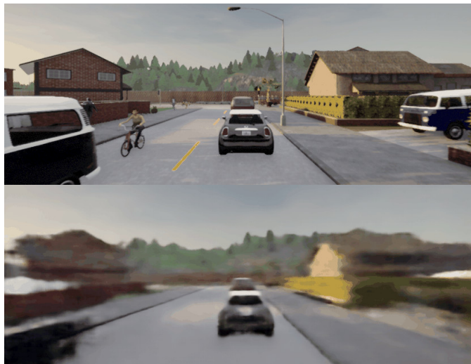
Fig. 1. The bottom row shows a scene reconstruction of a world model [6]. Compared to the ground truth, the model cannot recover all scene components, such as the bicyclist. This phenomenon can be exploited through a clear definition of normality and targeted training to detect anomalies.
