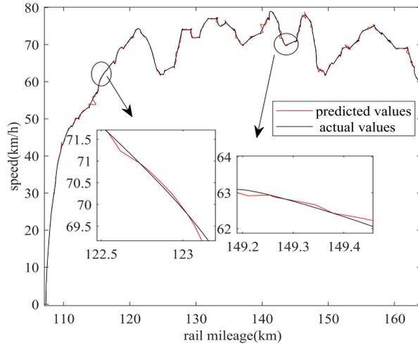
Figure 8. Speed trajectory prediction of the LSTMMH model.
