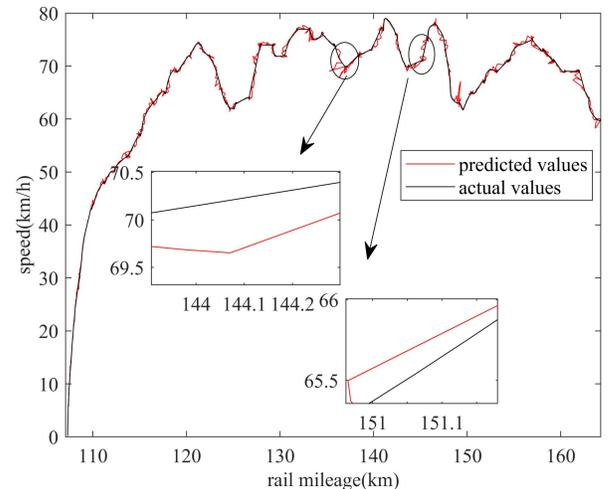
Figure 7. Speed trajectory prediction of the LSTM model.
