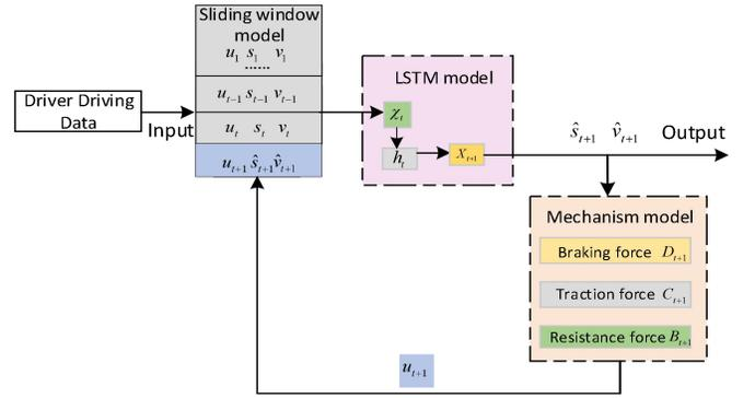
Figure 2. HHT mechanism-data hybrid model strategy.
