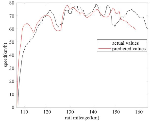
Figure 6. Speed trajectory prediction of the mechanistic model.
