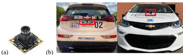
Fig. 7. Hardware set-up: a) Camera Sensor, b) cameras mounted in front and rear side of the testing vehicle.
