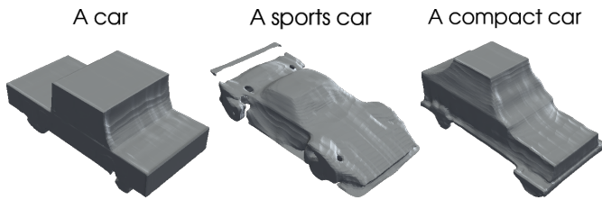
Fig. 1. Examples of car shapes generated using Shap-E based on the prompts “A car”, “A sports car”, and “A compact car”.
