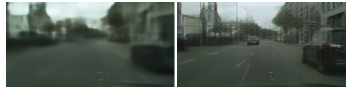
Fig. 7: Image reconstruction by a VAE with the latent space size of 512 \times 4 \times 4 and a \beta = 0.01 trained with (right) and without (left) the feature perceptual loss. Reprinted from [1].
