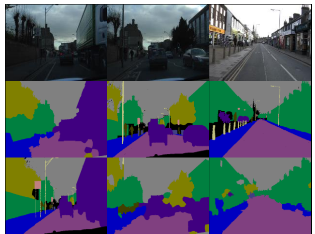
Fig. 6. Qualitative accuracy on the CamVid dataset is achieved by the PSO-optimised model. We presented a top-down, columnar strategy to show sample test images, ground truth annotation, and the segmentation model annotated images.
