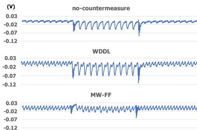
Figure 7 Comparison of the shapes of power consumption waveforms (traces)
