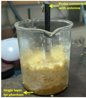
Fig. 9: Antenna in single layer fat phantom
