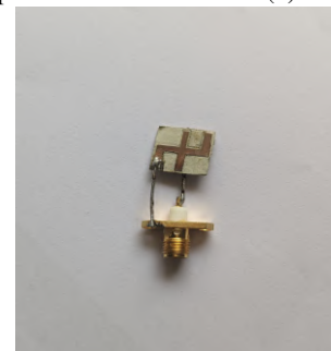
(c) Antenna connected to SMA
