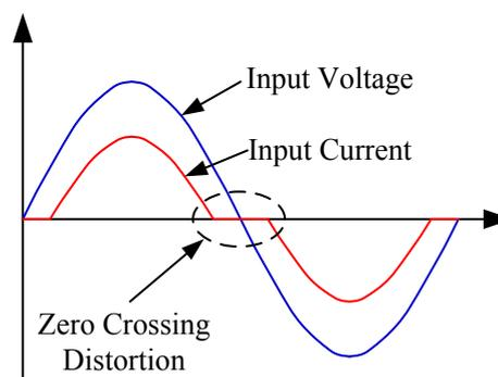
Fig 1. Input current distortion of PFC buck converter.
