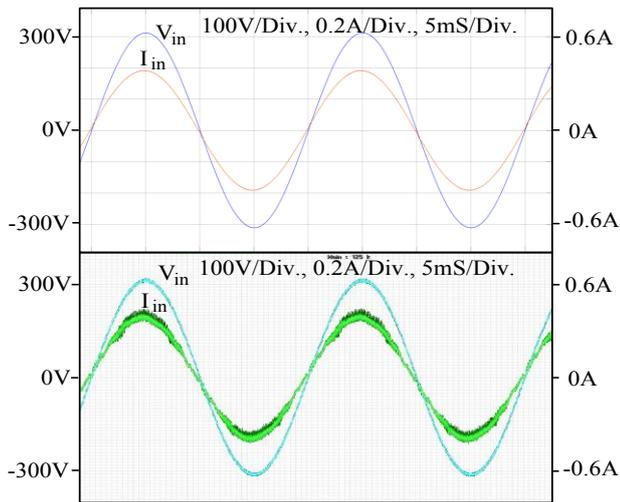
Fig 8. Input current and input voltage waveform of interleaved converter from the simulation and the experimental.
