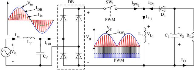
Fig 2. Conventional buck-boost PFC converter.
