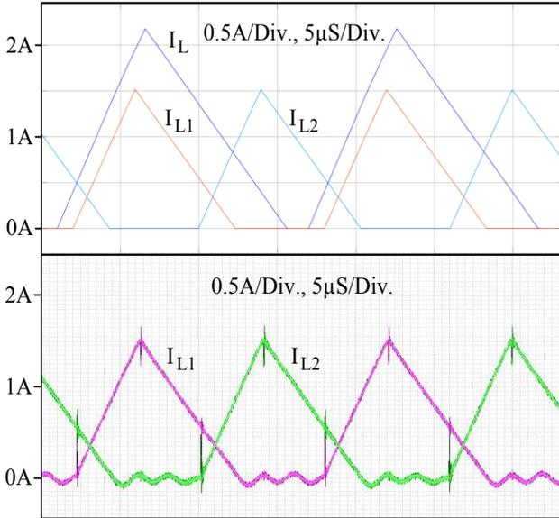
Fig 6. The simulation result of inductor current of conventional converter ( $I_L$ ) compares with inductor currents of interleaved converter ( $I_{L1}$  and  $I_{L2}$ ) and the waveforms of inductor currents of the interleaved converter prototype.
