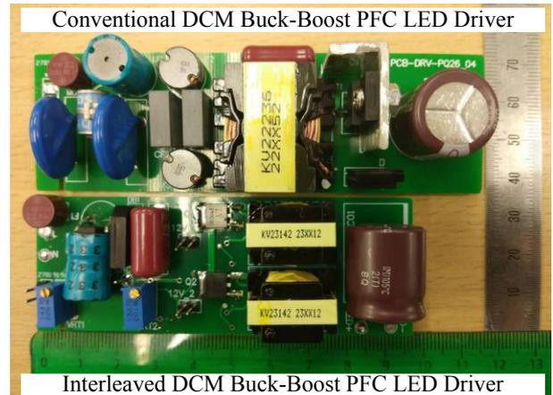
Fig 10. Photograph of conventional and interleaved Buck-Boost PFC LED driver prototype.
