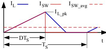
Fig 3. Waveforms of inductor filter current and switch current.
