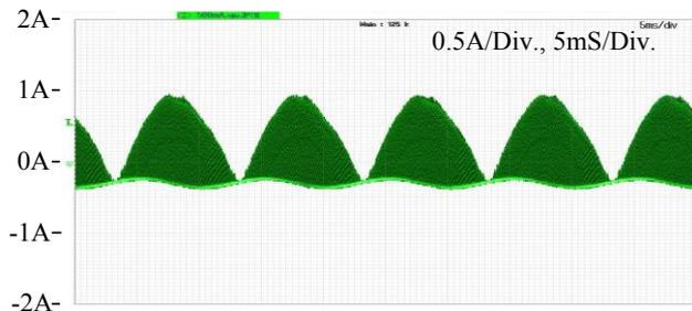
Fig 9. Low frequency output capacitor ripple current waveform.
