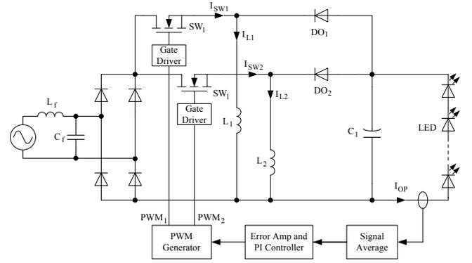
Fig 4. Proposed interleaved DCM buck-boost PFC LED driver.
