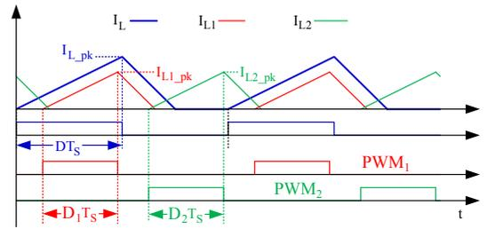
Fig 5. Comparison of inductor current of the conventional buck-boost ( $I_L$ ) converter and the interleaved buck-boost converter ( $I_{L1}$  and  $I_{L2}$ ).
