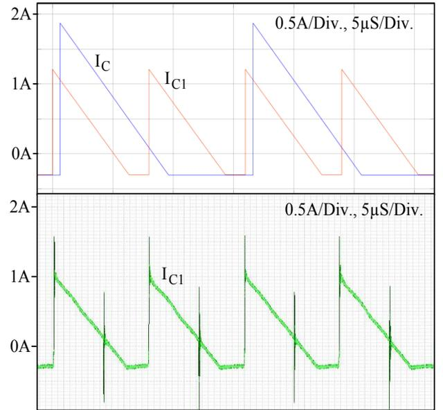
Fig 7. Output capacitor ripple current of conventional converter ( $I_C$ ) compares with capacitor ripple current of interleaved converter ( $I_{C1}$ ) and the ripple current waveform ( $I_{C1}$ ) of the prototype.
