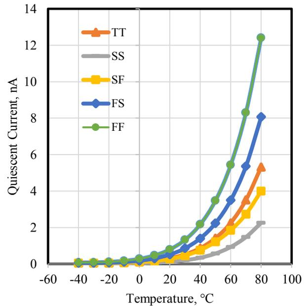
Fig. 6. Corner Simulation of the Proposed ZCD
