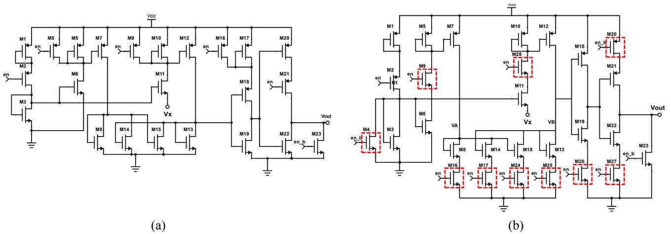
Fig. 2(a). Conventional ZCD; (b). Proposed ZCD
