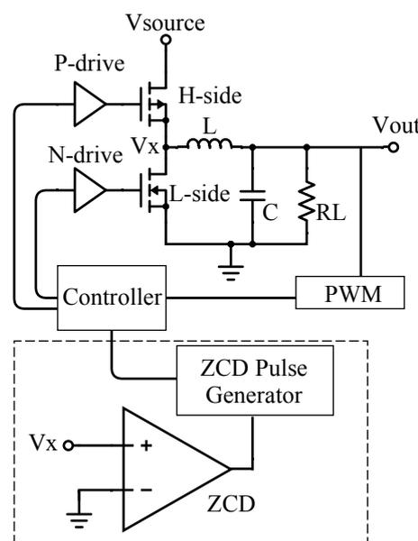
Fig. 1. DC-DC Buck Converter with ZCD
