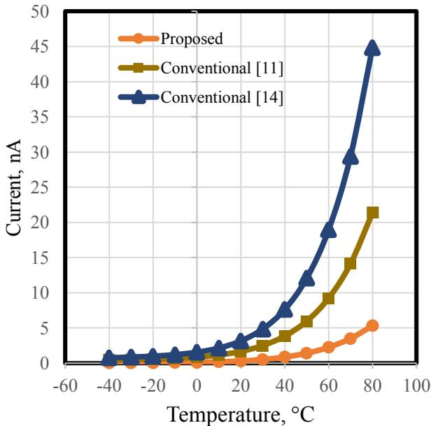
Fig. 5. Quiescent Current vs Temp Plot of Conventional and Proposed ZCD
