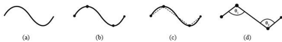
Fig. 2. Visual demonstration in determining the angle parameter used in the metric proposed in this research. (a) This is the original curve. (b) The sample points where the calculated gradient sign changes were considered
