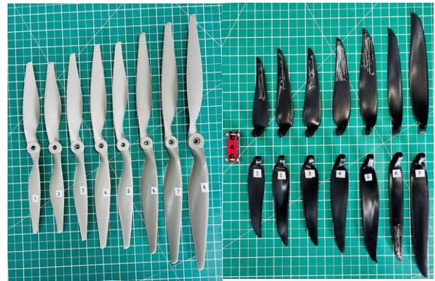
Fig. 1: The fixed propeller (left) and folding propeller (right) used for the experimental work
