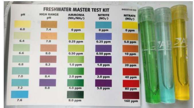
Fig. 2. Comparing the results of the ammonia, nitrate, and nitrite test to the color chart.
