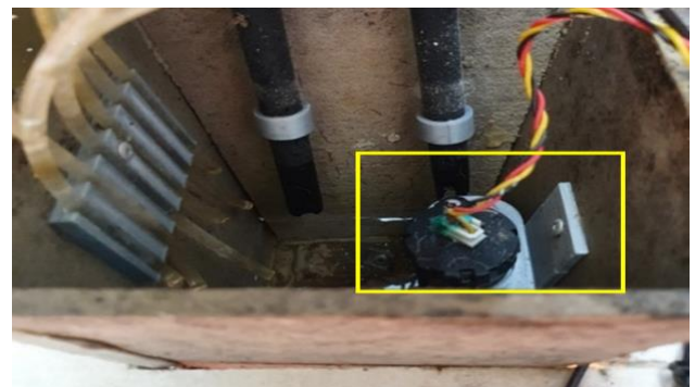
Fig. 3. Turbidity Sensor in the Sensory Chamber
