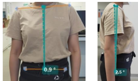
Figure 4. Determination of lateral trunk bend angle (left) and trunk inclination angle (right) using Kinovea, based on the markers placed.
