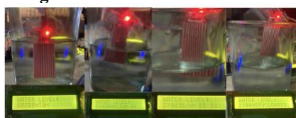
Figure 5.5. Water level sensor Calibration
