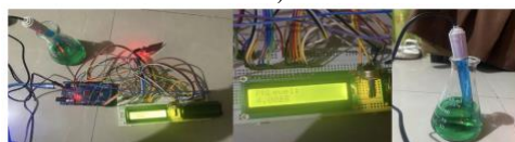
Figure 5.4. PH sensor Calibration
