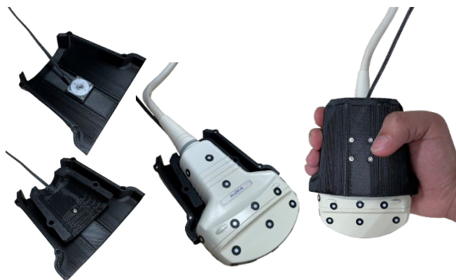
Fig. 3. The custom handle enabling the probe contact force measurement is designed to closely resemble the shape of the original ultrasound probe. The Tec Gihan's USL06-H5 three-axis force sensor is installed on the outer shell. The cover of the inner shell is mounted on the top surface of the force sensor. The ultrasound probe is placed inside the inner shell. The force sensor is the single-point contact between the shells designed with adequate clearance for the accurate force measurement.
