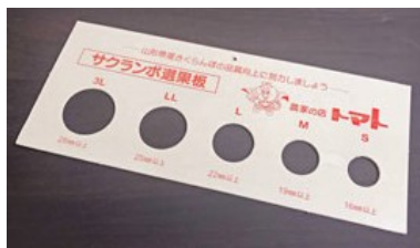
Fig. 1. Example of a reference plate for manual size sorting of cherries.
