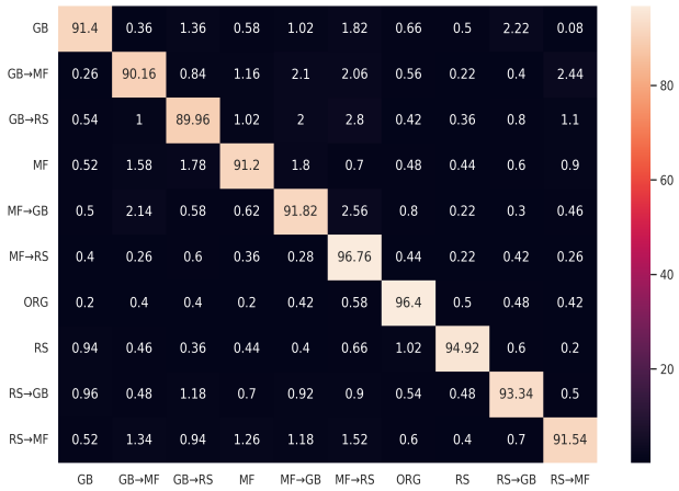
Fig. 5: Confusion matrix to identify operator chain detection (i.e. JPEG-series of manipulations-JPEG) with the proposed framework.
