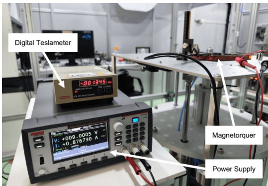
Fig. 4. The magnetic field measurement of the magnetorquer was done using a Group3 DTM-130 digital teslameter and supplied power from 0V to 15V.
