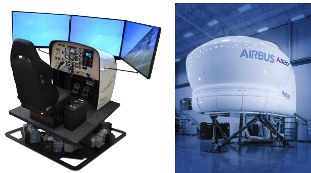
Fig. 1 Left: static flight training device by CKAS ( ckas.com.au ). Right: full-motion flight simulator at Airbus ( flightsafety.com ).
