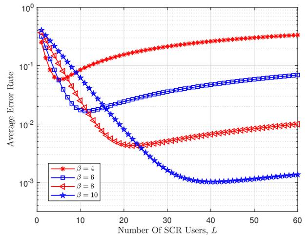
Fig. 3. Average error rate versus  $L$  for the proposed CR network using the SSI fusion rule for various  $\beta$  values,  $\zeta_s = 10$  dB.
