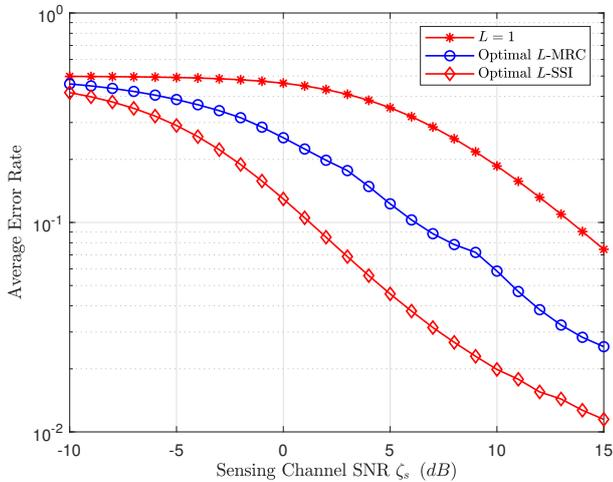
Fig. 5. Average error rate versus  $\zeta_s$  in dB at  $\beta = 5$ , Optimal  $L$ .
