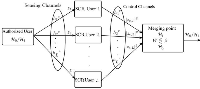
Fig. 1. Schematic representation of spectrum sensing in the CR network using the selective soft-information fusion scheme.
