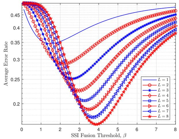
Fig. 2. Average error rate versus  $\beta$  for the proposed CR network using the SSI fusion rule for various values of  $L$ ,  $\zeta_s = 2$  dB.
