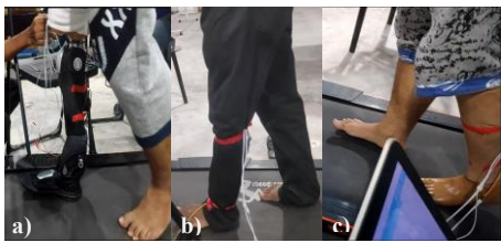
Fig 8 : Hardware implementation and 3-way data collection: a) With Prosthetic Exo-leg, b) Healthy human walking, & c) With poly acrylic leg
